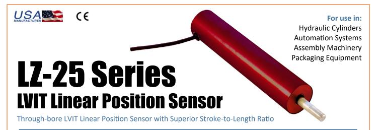
The LZ-25 Series of LVIT (Linear Variable Inductance Transducer) position sensors are contactless devices designed for frictionless measurement in factory automation or assembly machinery applications where space is a premium, as well as for external mounting on hydraulic cylinders to sense rod position.
