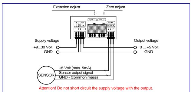
No problem with GND - all at same potential, even in mulitaxial systems! The sensor supply voltage (+5V, max. 5mA) can (because of the high accuracy) be used as reference voltage for subsequent electronics, e.g. OPV or ADC.
